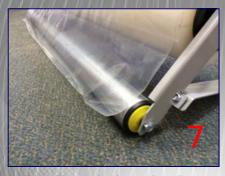
Pull out film to the front of applicator with the adhesive side facing Outwards.
