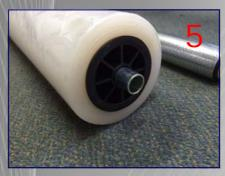
Insert end caps x 2 into Core of film roll exposing hollow bar
