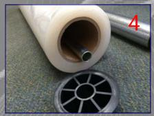
Insert Hollow bar through selected film roll chosen
